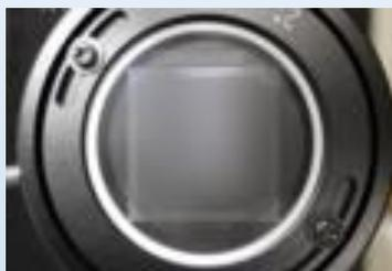
DOE: Diffractive Optical Element (回折光学素子)
